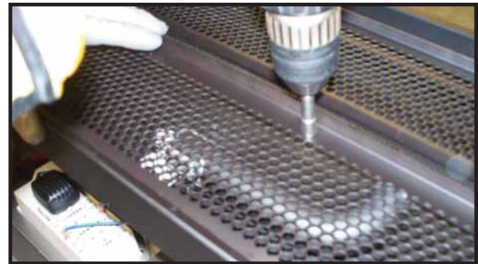
Figure 12.9 Removing Screws from Base Pan.
